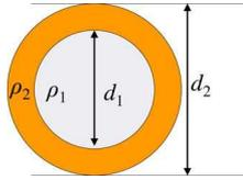
Fig. 4. Conductor comprising two concentric cylinders of different metals. In the case of CCA (copper-clad aluminum), the outer cylinder, with resistivity  $\rho_2$ , is copper and the inner cylinder, with resistivity  $\rho_1$ , is aluminum.
