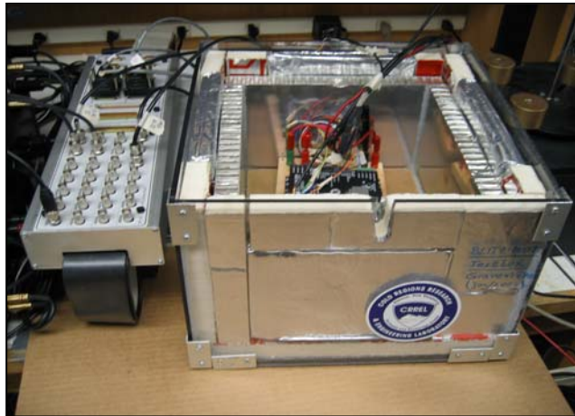
Figure 3.27: dSpace and Test Box with Compon. inside
