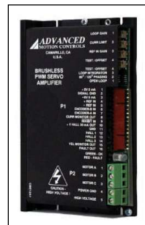
Figure 3.10: Motor Controller [AMC]
