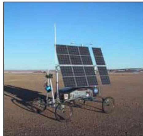
Figure 2.7: Hyperion with vertical solar panel [SHA01]
